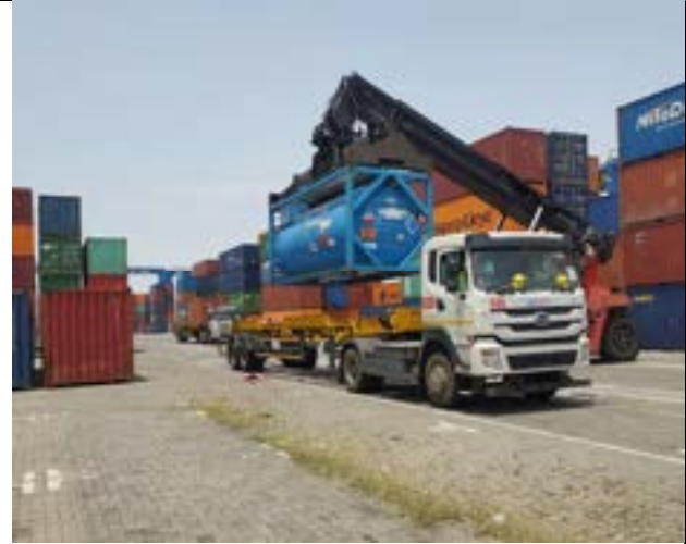
Container taken to leak bund by reach stacker
